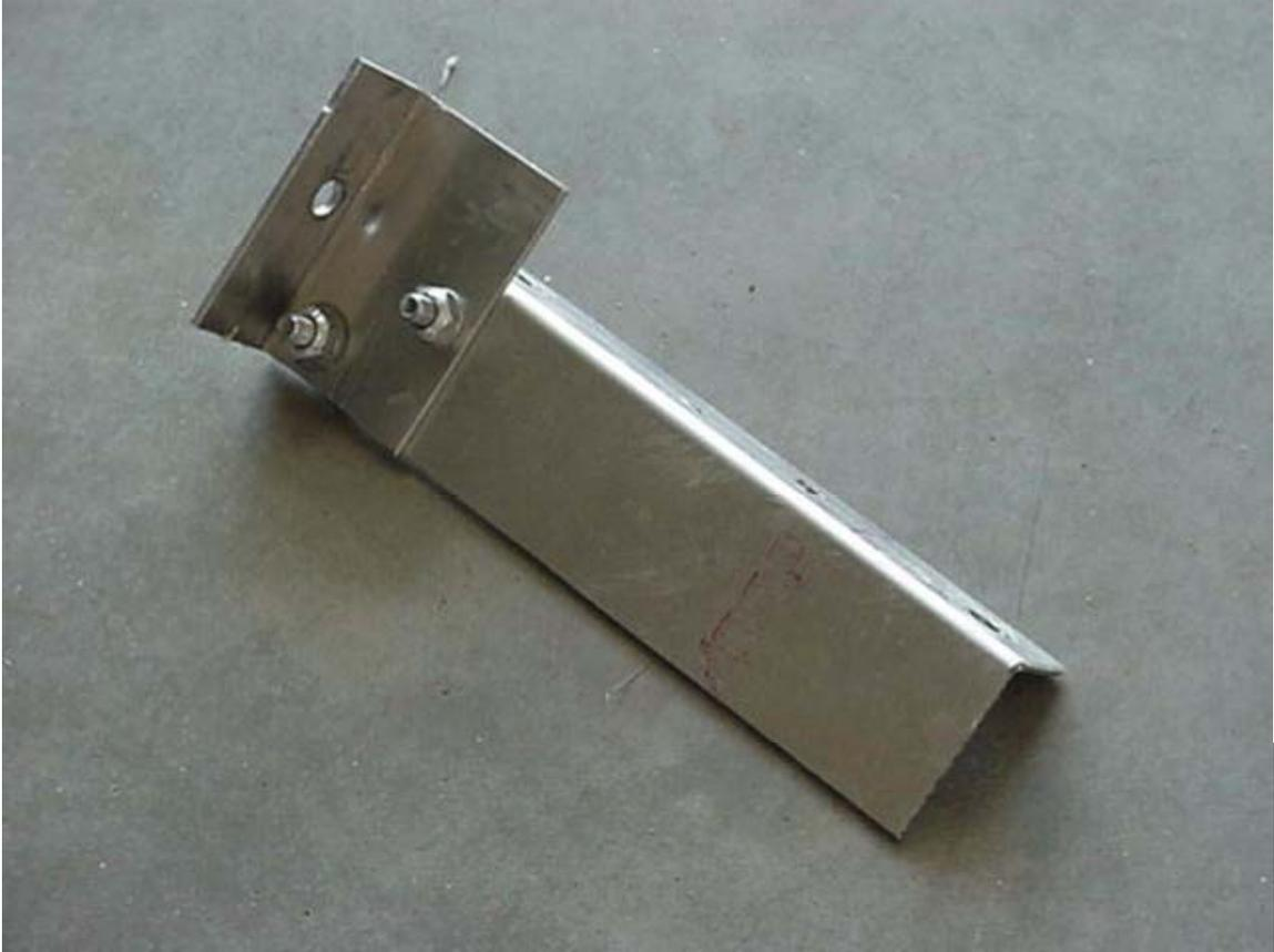
**Figure 2. Throttle bell-crank mounting bracket**
