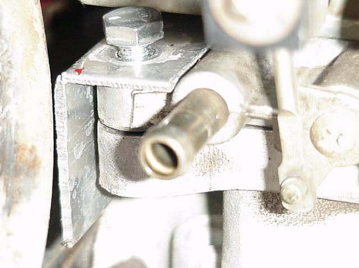
**Figure 3. Throttle bell-crank mounting bracket side view**
